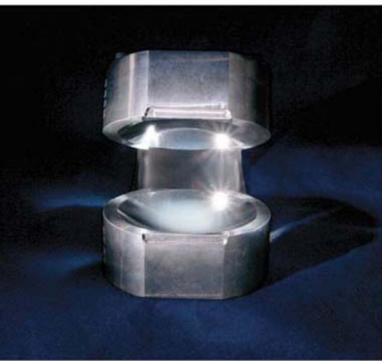
Quantum resonator. Two mirrored half-sections are opened to show the interior of a high-quality microwave cavity. Such storage chambers are used to control and study the interaction between single atoms and single photons.
